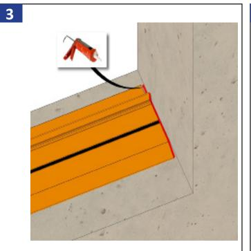
Apply sealant to both ends of the sill flasing to the center post and wall framing to create an end dam.
