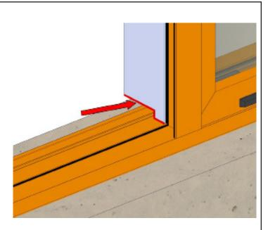
Cut T-Mull to match window height and notch at the sill (1/2 x 2 3/4) to clear the interior leg of the sill flashing.
