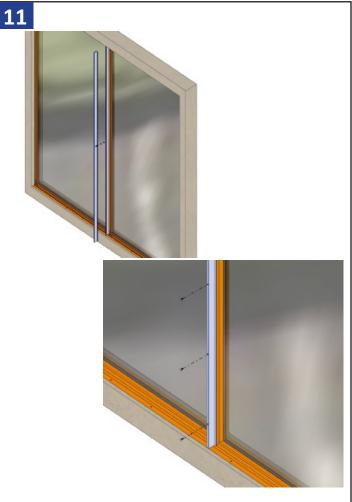
Install the T-Mull base plate using bolts provided by QWP.
