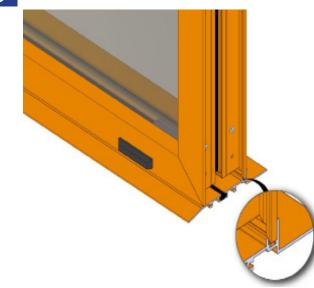
Install the first window in the continuous bead of sealant and use the snap trim clips provided.
