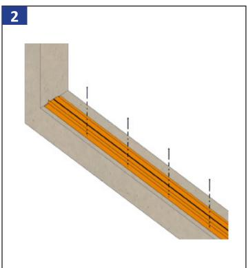
Set sill flasing on the continuous bed of sealant. Install through the interior anchor leg using fasteners supplied by the insaller.
