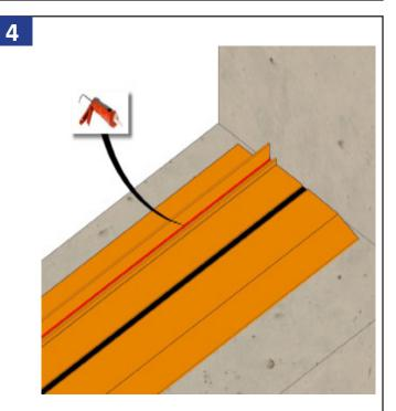
Apply a continuous bead of sealant into the track where the inside window leg will rest.
