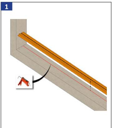
Apply Continuous bead of sealant which the sill flashing will set on.
